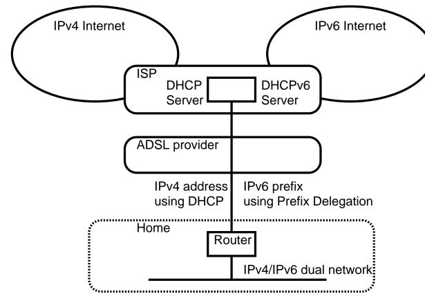
The router at home can be considered to be connected ISP's Ethernet network
