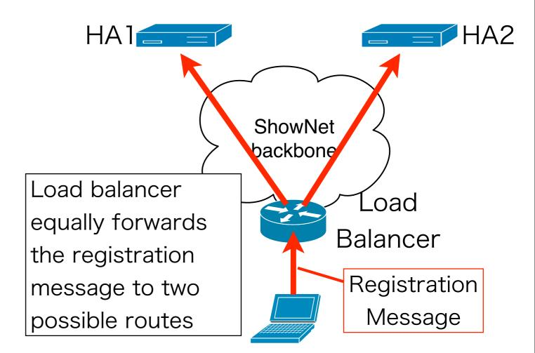
1.Mobile layer need to coordinate with underlaying routing layer 2.Load balancer must have knowledge of Mobility protocols
